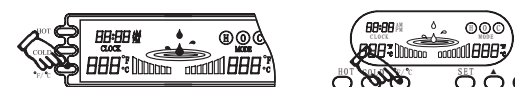
5. Press °F/°C key to switch between temperature display; default temperature is set in°C.
